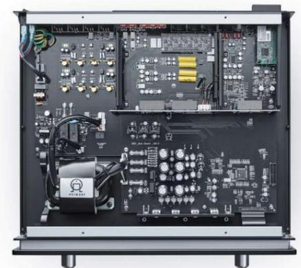
The inside of a completely analog PRE35, without both DAC and Prisma cards. In principle, consistently surface-mounted also here (SMD). Note the R-core transformer in the lower left corner of the image, which Technics was early to use, with even lower electromagnetic radiation than a ring-core transformer.
