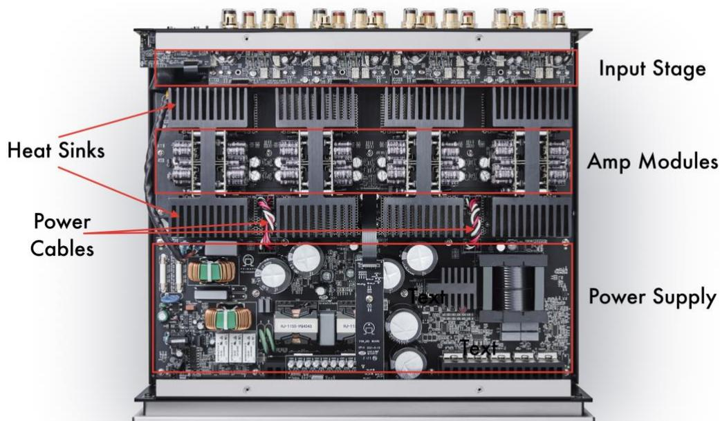
The modular design of the heatsink and paired output circuits assembly, utilize a multi-pin connector and secured by four screws, allowing for easy field replacement should service be required.
