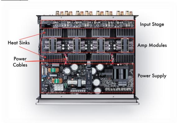
The modular design of the heatsink and paired output circuits assembly, utilize a multi-pin connector and secured by four screws, allowing for easy field replacement should service be required.
