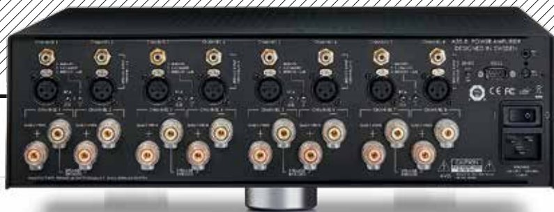
ABOVE: Arranged in four stereo banks, each amplifier 'module' has XLR and/or RCA inputs (selected via toggle switches) and may be bridged to form higher-power single-channel outputs. Auto signal sensing, trigger and RS232 control is included
