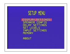
Use the INPUT SELECTOR on the front panel or the ▲ and ▼ buttons on the remote control to highlight the SPEAKER CONFIG option and press the SELECT button on the front panel or remote control to select it.
