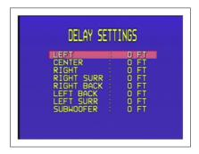
Highlight each of the speakers in turn, using the INPUT SELECTOR on the front panel or the ▲ and ▼ buttons on the remote control, and use the VOLUME control on the front panel or the ◀ and ▶ buttons on the remote control to adjust the delay.
