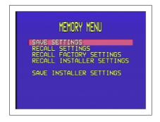
Highlight SAVE SETTINGS and press the SELECT button on the front panel or remote control to select it.
