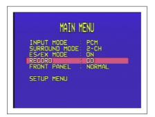
Alternatively, select **NORMAL** to make the record outputs follow the currently selected source, or **OFF** to mute the record outputs.
