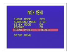
The front panel will also be unlocked if you switch off the SP31.7 and switch it on again.
