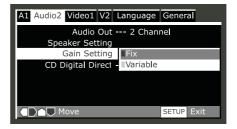
When set to 'Variable', the overall output level may sound quieter than when set to 'Fix'. This is not a malfunction.
