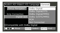
All options (except Not Connected) assume PCM compatibility. The PCM option means only compatible with PCM. Consult the manual that came with your amplifier if you're unsure about compatibility with any of these formats.
