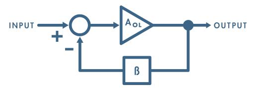
The UFPD amplifier actively adapts the loop gain to keep the total loop stable during start up, clipping and current limit. It senses the changes to the filter output and compensates by applying the precise amount of feedback. This adaptive control allows for several more dBs of constant loop gain across the audio band and maintains performance irrespective of load (impedance) variations.
